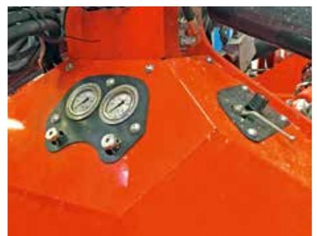
The OPTIMER 6000 and 7500 stubble cultivators are equipped with the optional STEADY CONTROL ground tracking system. It is fitted as standard on the 9 and 12 metre models for perfect control of the working depth whatever the soil conditions
