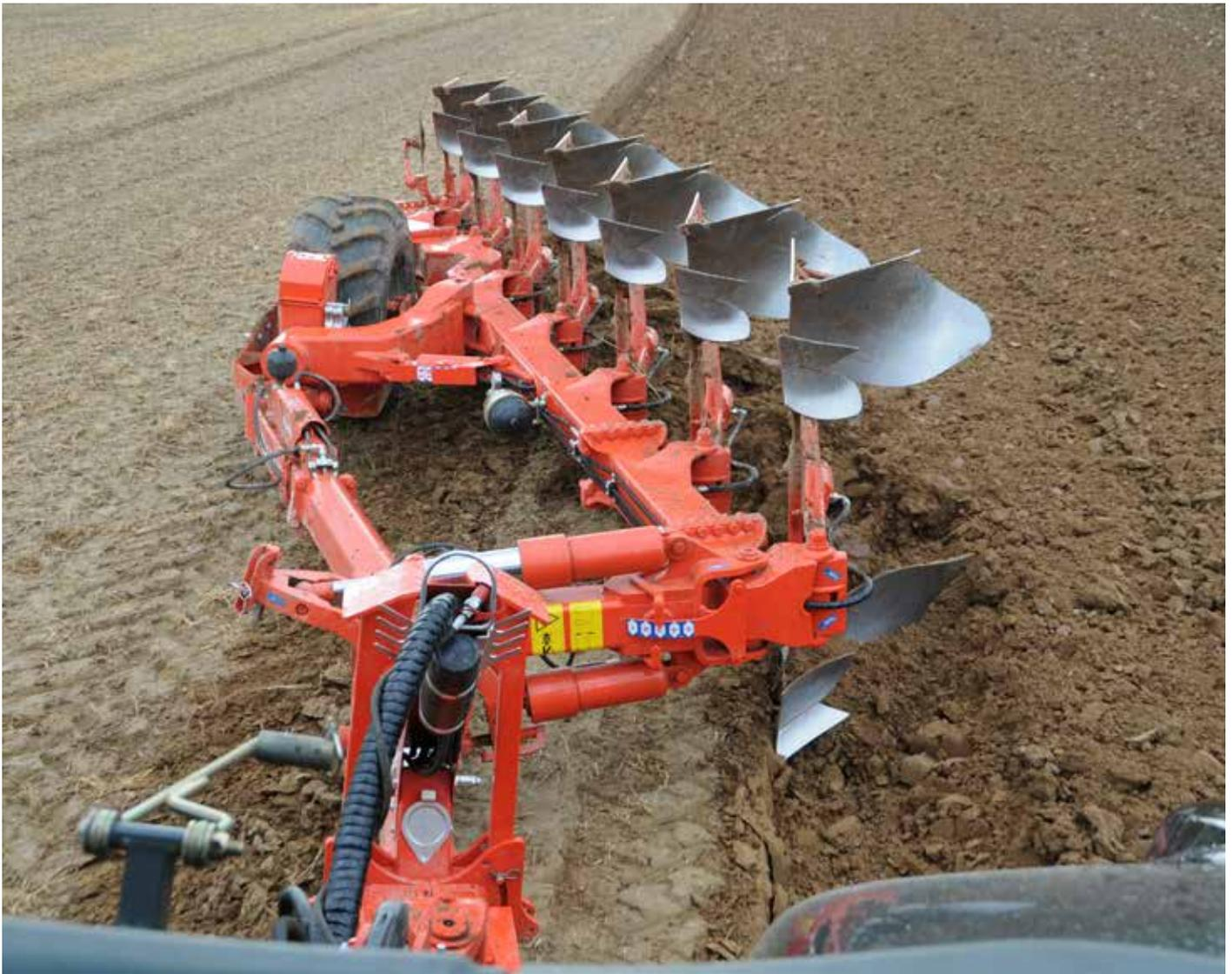
For additional serenity, this variable width system is maintenance-free. All pivot points are stopped from rotating and fitted with bushes.
