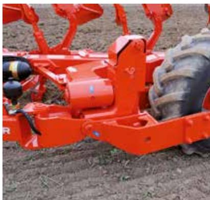
**5.** A large sized wheel (500 x 1000 mm or 500 x 1200 mm) supported on both sides ensures stability in U-turns and provides a longer hub life !!
