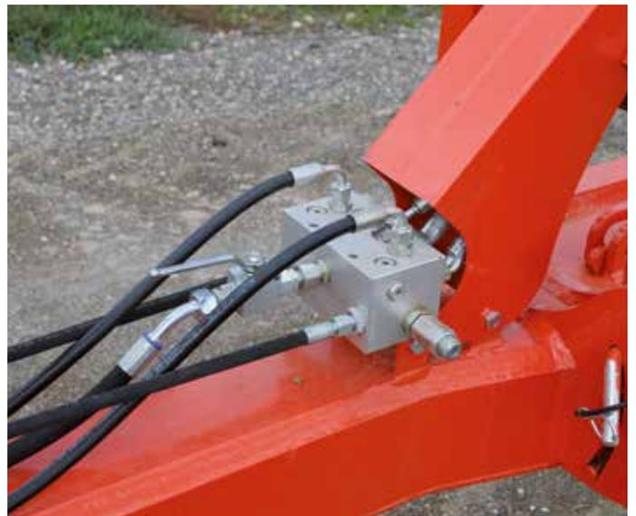
For your comfort : fewer spool valves to operate in U-turns as the entire range is equipped with hydraulic sequencing as standard.
