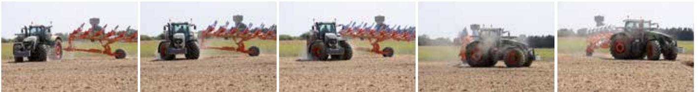
With sufficient space between the headstock and the first point, there is no risk of damaging the tractor, even in the sharpest U-turns.
