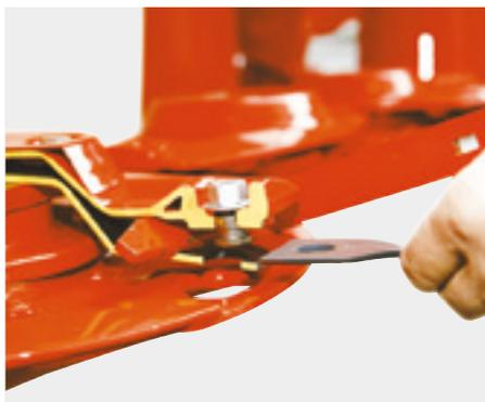
Replacing a FAST-FIT knife quickly
