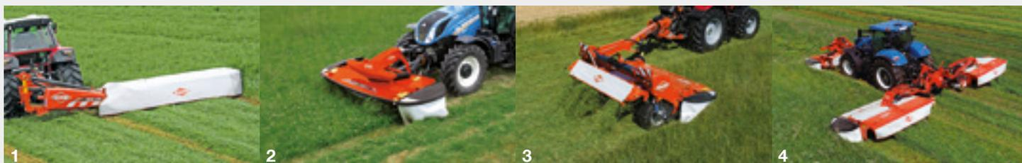
1. Rear-mounted mowers - 2. Front-mounted disc mowers - 3. Trailed disc mowers - 4. Triple gang disc mowers
