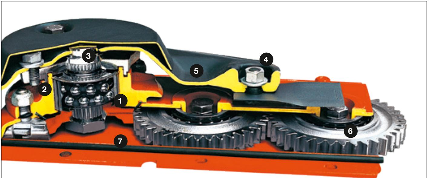
**1. Withstands the highest loads:** special high-capacity bearings fitted in anti-distortion housings.
