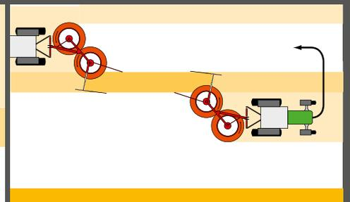
Double swath raking, working width 600 cm (19'8")
