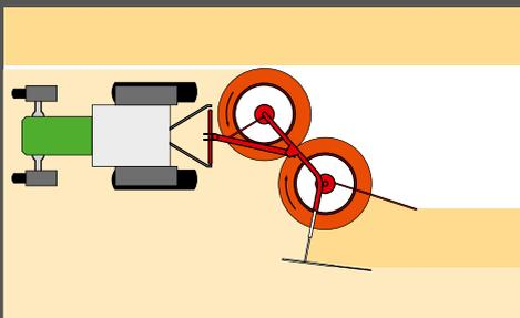
Single swath raking, working width 360 cm (11'10")
