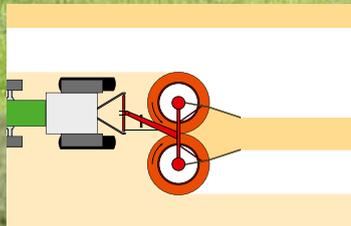
Single swath raking, working width 300 cm (9'10")
