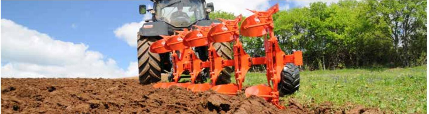
The MASTER 153 ploughs have been designed to meet the same requirements as the 123 series, but are designed for more intensive use and more difficult working conditions with more powerful tractors ranging from 95 to 270 hp. This range is available in MULTI-MASTER and VARI-MASTER versions, with safety traction bolts or Non Stop Hydraulic safety, from 4 to 6 bodies. Possibility of mounting helical-bodies for easy passage of wide tyres.
