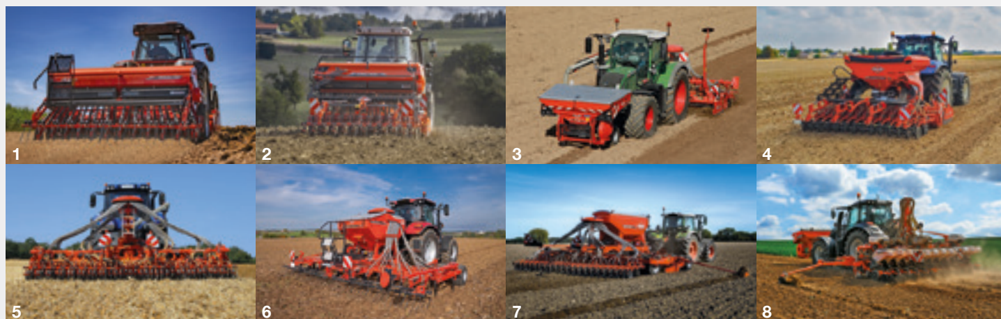
1. Mounted mechanical 2. Integrated mechanical 3. With front hopper 4. Integrated pneumatic 5. Folding pneumatic 6. Mounted min-till 7. Trailed min-till 8. Precision seed drills.
