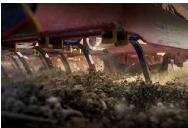
Carefully selected raw material and design, ensures peak performance and depth precision of the Extreme tines.
