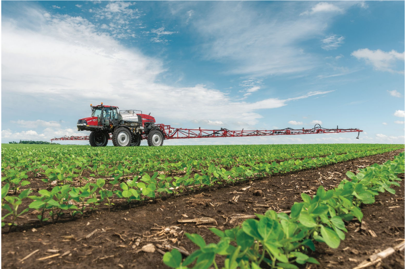
New AutoBoom® XRT automatic boom height control, available on Patriot® series sprayers, is designed to increase the accuracy and coverage of applications.
