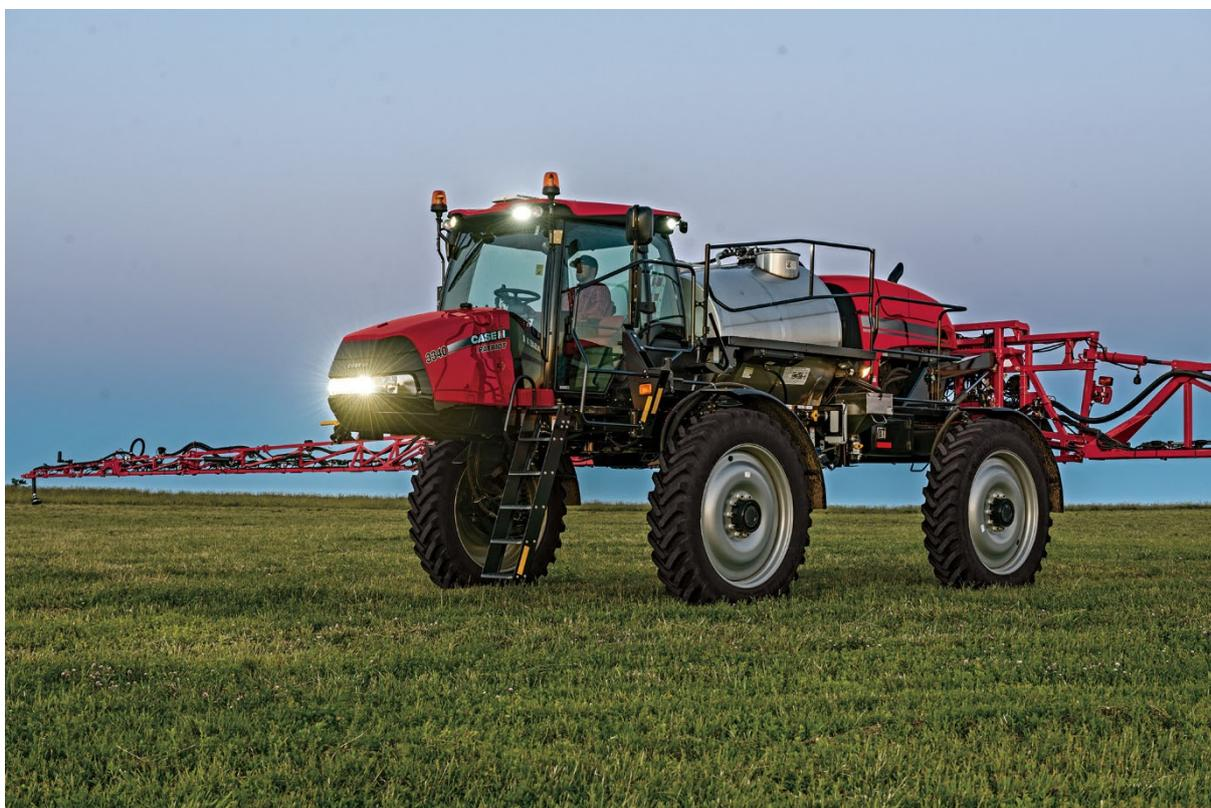
*AFS AccuTurn™ Automated headland-turning technology is now available on Case IH Patriot series sprayers, offering operators improved accuracy and reduced fatigue during chemical applications.*
